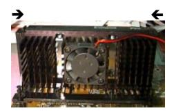
Insert the Processor like inserting a PCI or an ISA card.
